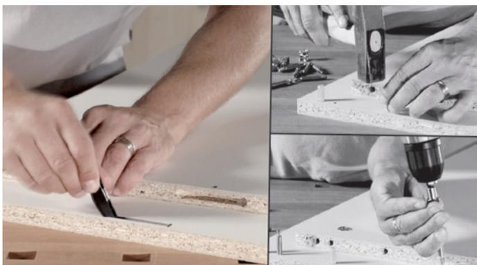
The advantages compared with conventional excentric solutions: the P-System (left) connectors can be inserted tool-free in the bench room or outside the workshop. The small access hole scores points visually.
