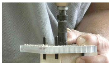
2. Drill the table legs Apply on the edges without measuring or marking
