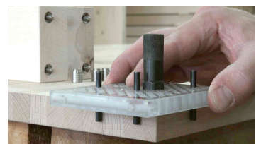
4. Drill the table top Apply with the same position of the pins with- out measuring or marking
