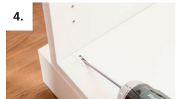
4. Join furniture elements with cordless screwdriver and Cabineo tool. Easy, fast working with preset torque about 2.5 Nm
