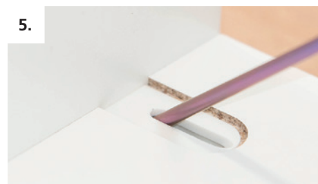
Join the workpieces with a cordless screwdriver (torque about 2.5 Nm)
