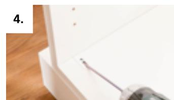
**4.** Join furniture elements with cordless screwdriver and Cabineo tool. Easy, fast working with preset torque about 2.5 Nm
