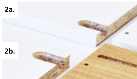
Machining the workpiece, including milling the contour for the cover cap
