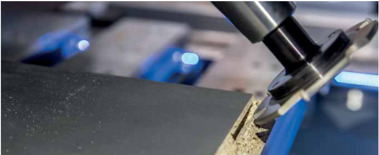
P-System profile groove machining with Homag Venture 316 L CNC 5-axes
